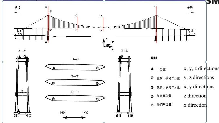
Figure 1 Accelerometer locations and directions for the instrumentation network on the Pearl River Huangpu Bridge
