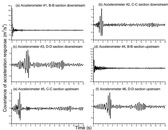
Figure 2 - the covariance of the acceleration responses with reference to Accelerometer #1
