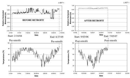
Figure 3. Relative horizontal movement measured at Beam 6 in Span 117.
