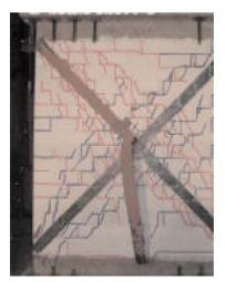
Figure 2. Numerical/Experimental comparison. Smeared Crack plot (D\_100) vs. experimental pattern.
