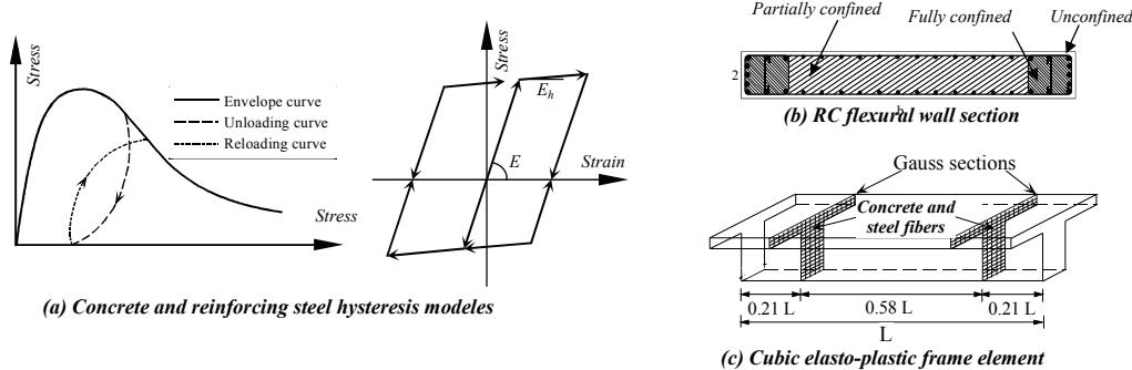
Figure 2. Ingredients of the ZEUS-NL (Elnashai et al., 2010) fiber-based models: (a) material models, (b) sample of concrete sections, and (c) elasto-plastic frame element.
