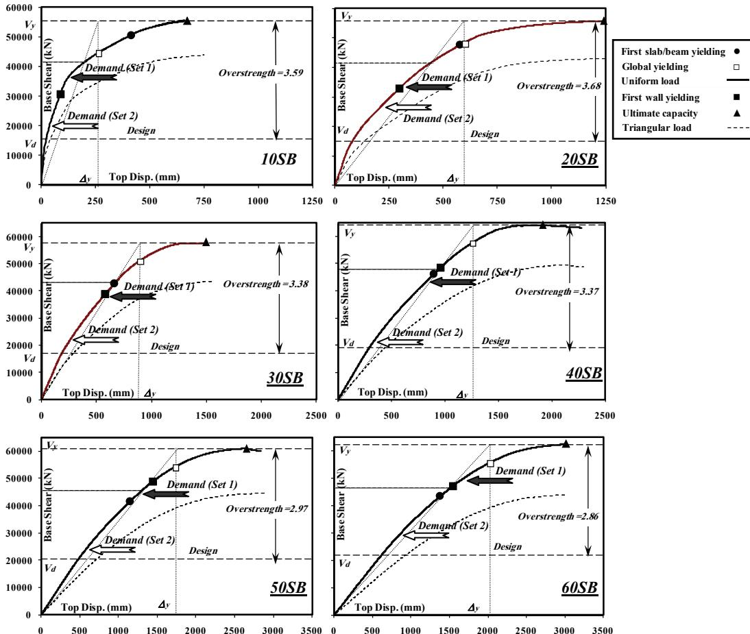
Figure 3. Capacity envelopes of the reference structures in the transverse direction along with seismic demands from two seismic scenarios at the design PGA.
