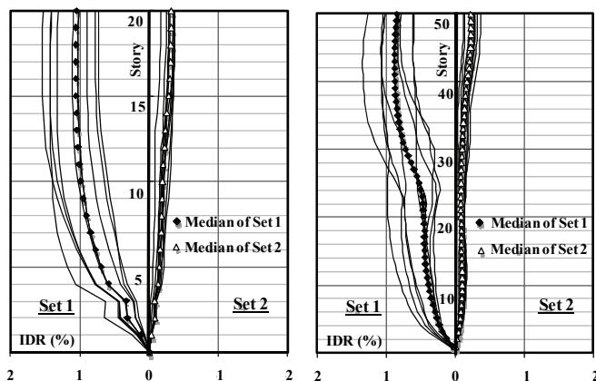
Figure 4. Maximum and median interstory drift of the 20 and 50-story buildings at twice the design PGA from two earthquake scenarios.
