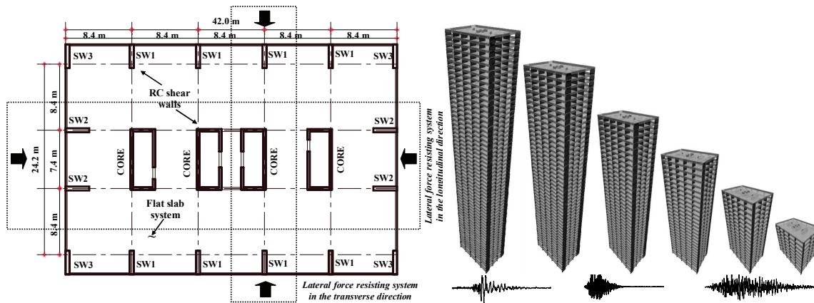
Figure 1. Three-dimensional analytical models used in design along with the building layout, which shows different lateral force-resisting systems in the longitudinal and transverse directions.
