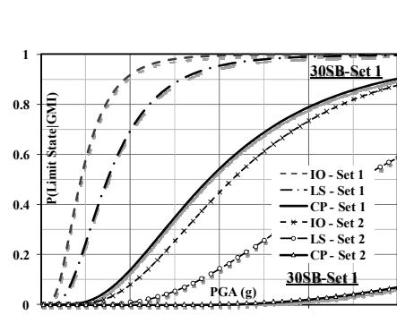
Figure 5. Vulnerability curves of the 30-story building obtained from IDCAs using two seismic scenarios.
