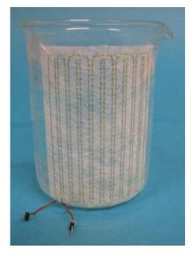
Figure 5: Possible sensor geometry with a capacity of 100 pF
