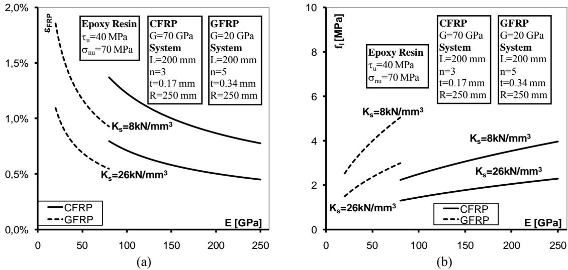
Figure 5. Influence of FRP elastic modulus on: (a) FRP hoop strain; (b) confinement lateral pressure.
