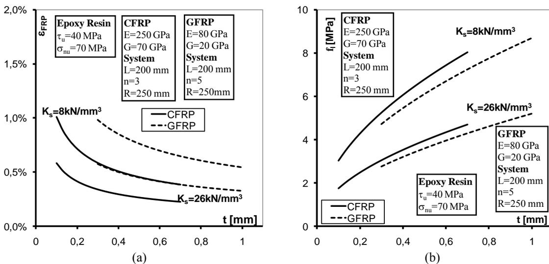
Figure 1. Influence of FRP thickness on: (a) FRP hoop strain; (b) confinement lateral pressure.
