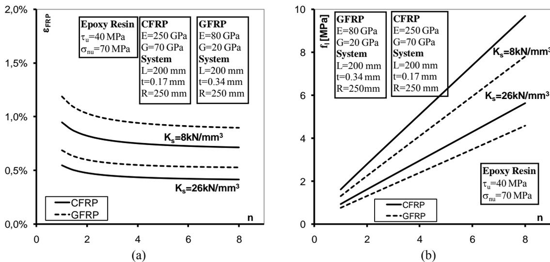
Figure 3. Influence of number of FRP layers on: (a) FRP hoop strain; (b) confinement lateral pressure.
