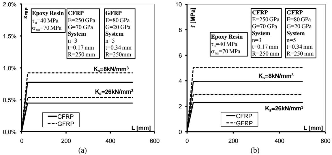
Figure 2. Influence of FRP anchoring length on: (a) FRP hoop strain; (b) confinement lateral pressure.
