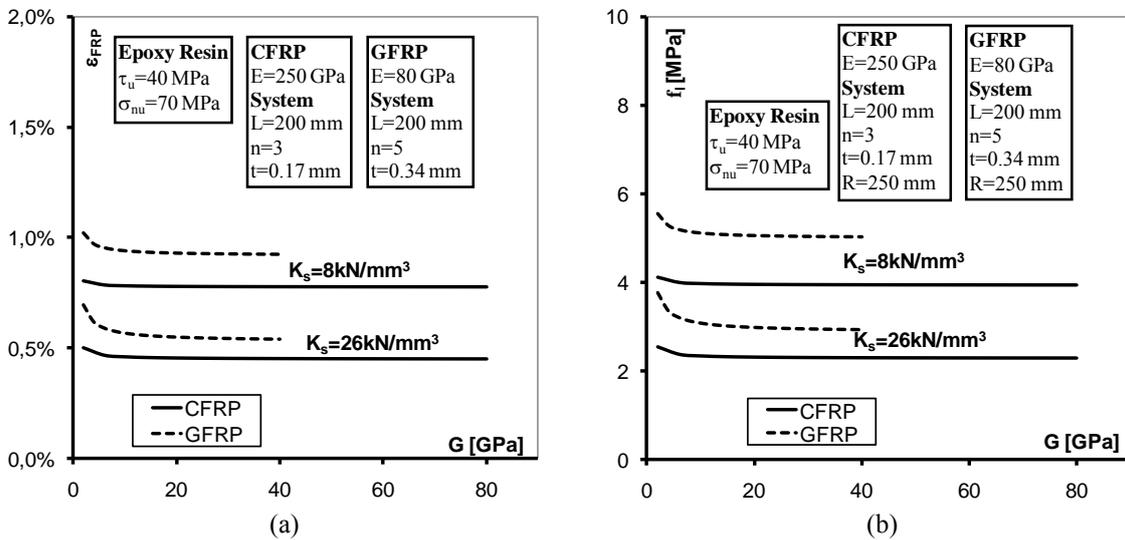
Figure 4. Influence of FRP shear modulus on: (a) FRP hoop strain; (b) confinement lateral pressure.
