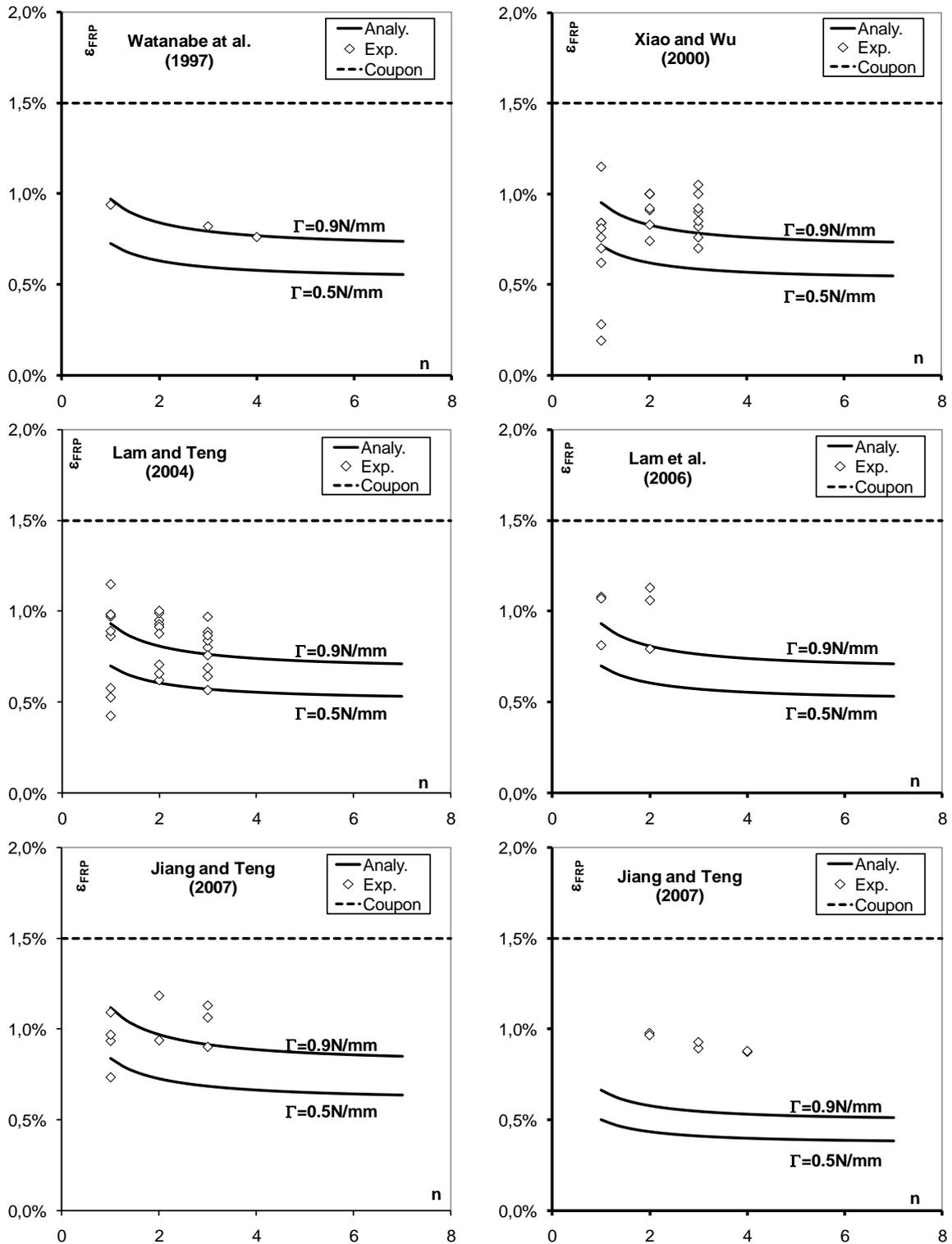
Figure 6. Experimental vs. analytical results on RC columns confined with CFRP jacketing.
