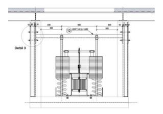
Figure 8, Complete TMD in steel cage beneath the deck plate.
