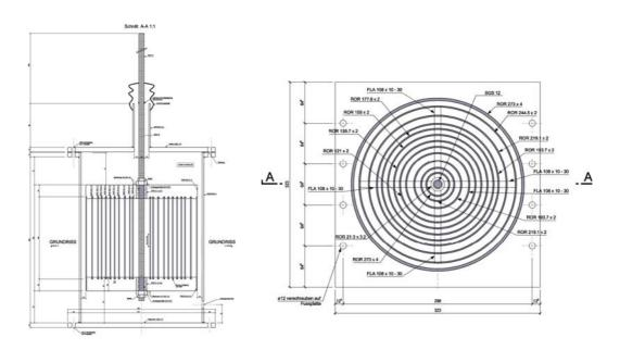
Figure 7, Viscous damper element (detail of the shop drawing).
