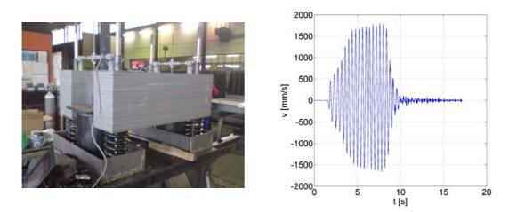
Figure 10, Workshop test, left: complete TMD, right: velocity decay of the damper mass
