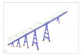
Figure 1, FE-model of the complete bridge
