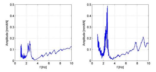
Figure 12, Frequency response of the bridge deck with (left) and without (right) TMD's.
