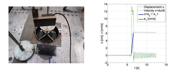
Figure 9, Damper element, test set-up, measured displacement and velocity (right)
