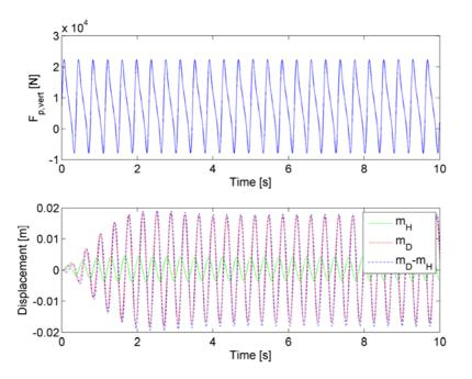
Figure 6, Runner's excitation for 10 second (top) and response of the TMD and the bridge deck (bottom),  $m_{\rm H}$ : mass of bridge,  $m_{\rm D}$ : damper mass
