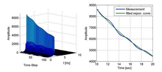
Figure 5, Short time Fourier transform of the velocity (left) and exponential decay (damping 0.9%, right).
