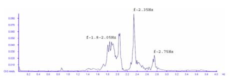
Figure 4, Measured amplitude function, vertical direction
