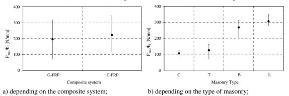
Figure 3. Maximum ultimate strength-per-unit-width observed in the pull-out tests.
