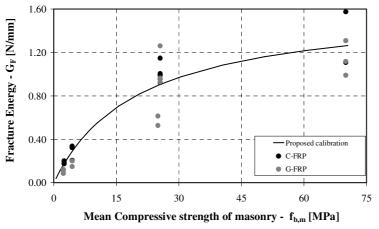
Figure 5. Fracture energy G<sub>F</sub> vs. mean compressive strength of masonry: proposed rational relationship
