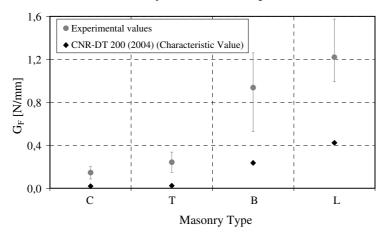
Figure 4. Experimental values and a possible theoretical prediction of fracture energy.
