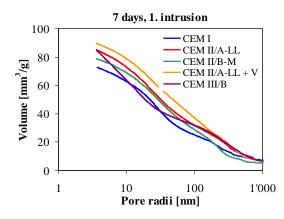
Figure 2: Total porosity and pore size distribution of mortar determined with MIP at an age of 7 days.
