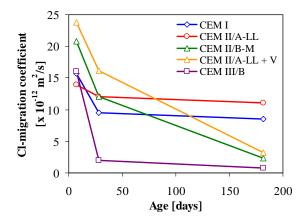
Figure 7: Chloride migration coefficient versus age.
