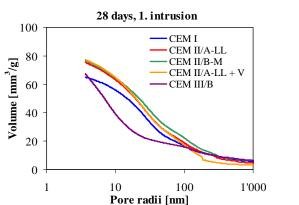
Figure 3: Total porosity and pore size distribution of mortar determined with MIP at an age of 28 days.
