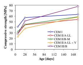
Figure 1: Compressive strength versus age.
