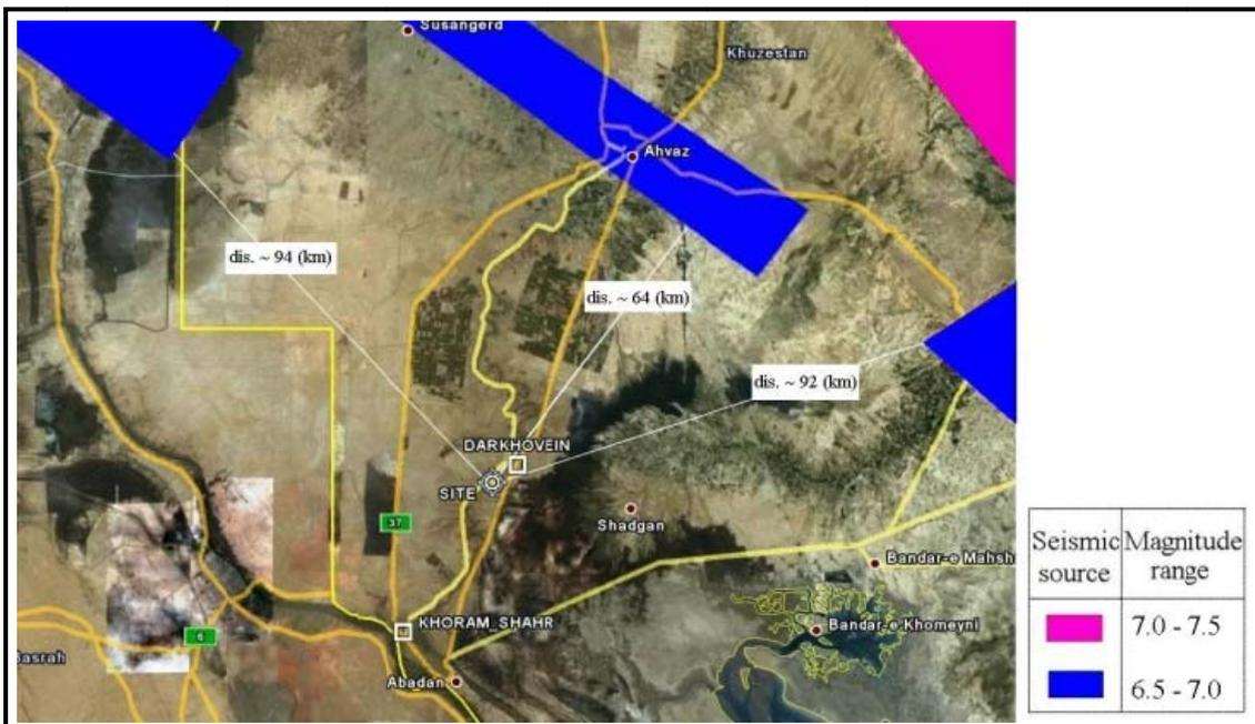
Figure 3. Earthquake sources around Darkhovein (source locations is based on Mirzaei et al, 1998)
