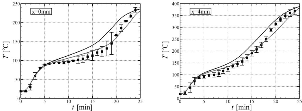
Figure 1. Comparison between HETRAN predictions, with (grey solid line) and without (black solid line) mass transfer, and experimental data (square symbols) [Ghazi Wakili et al. (2007)] of the temperature evolution inside the gypsum board.
