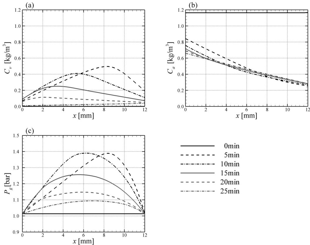
Figure 2. Spatial distribution of: a) vapor mass concentration, b) air mass concentration and c) mixture total pressure at different time steps.
