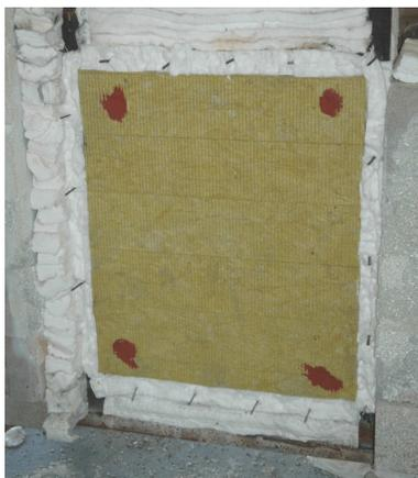
Figure 3. Insulated slab – Fire side.
