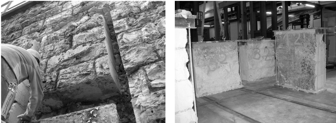
Figure 3: Removal of masonry object for a compression test
