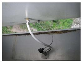
Figure 1: Wind Pressure sensor
