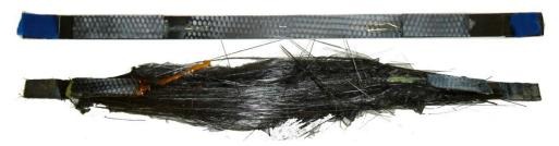
Figure 5 CFRP specimen 2.1, transient test, before and after the test.
