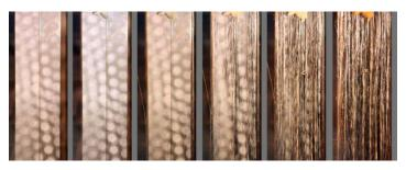
Figure 3 Damage progress during test for specimen 2.1. Temperatures are 28, 77, 183, 200, 210 and 256 °C from left to right.
