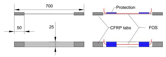
Figure 1: CFRP coupon dimensions and fibre optic sensor locations (all dimensions in mm).
