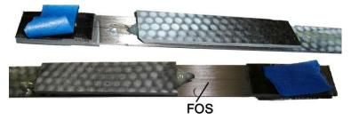
Figure 4 Fibre optic sensor and protective cover installation details.
