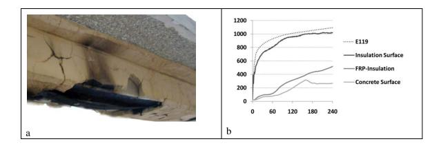
Figure 8 (a) Beams after four hours of exposure to standard fire and (b) Temperature (°C) vs. exposure time (min) at midspan of the T-beam.
