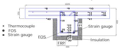
Figure 7 Details of reinforcement and instrumentation for beams (dimensions in mm).
