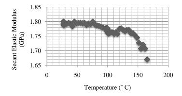
Figure 6 Secant modulus for specimen 2.1 vs. temperature.
