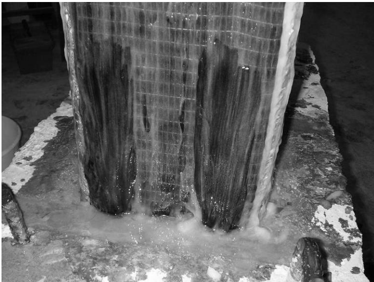
Figure 6. Anchorage in the foundation (Fyfe Company).
