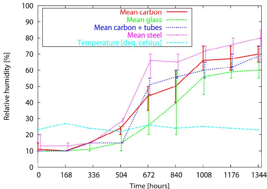
Figure 4. The results of additional moisture diffusion tests on insulating glass panels with spacers from carbon fibre epoxy (with and without tubes), glass fibre epoxy, and steel. The temperature at each determined relative humidity point is also shown. The first 4 weeks of thermal cycling between -18°C to 53°C was followed by a period of 7 weeks at a constant temperature of 58°C .
