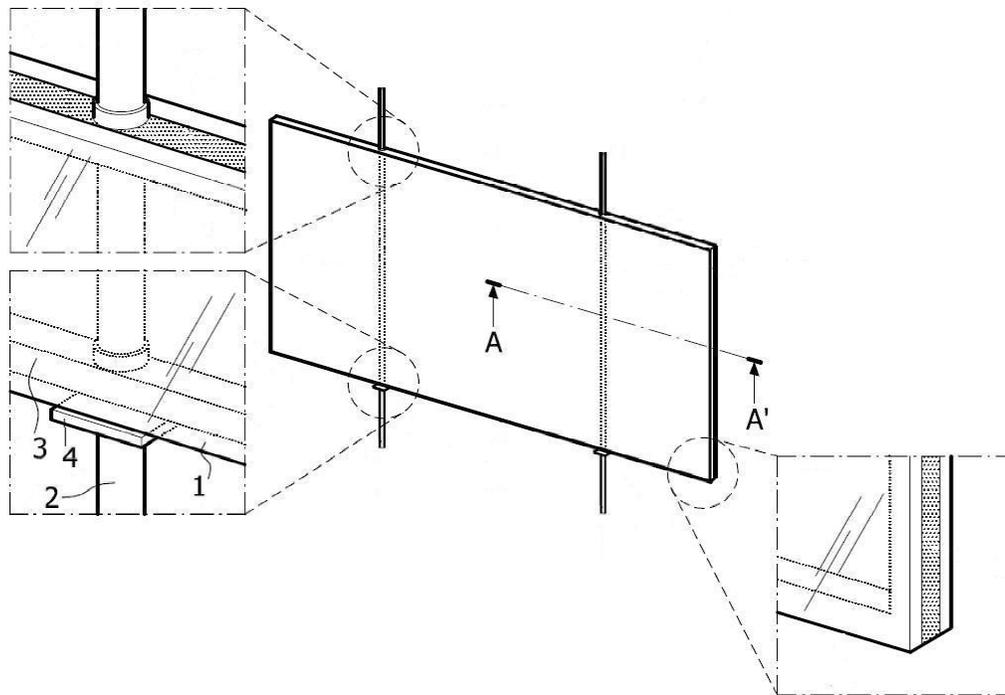
Figure 1. The developed and patented composite façade concept with (1) the glass plate, (2) the carbon fibre epoxy tube, (3) the carbon fibre epoxy spacer, and (4) the carbon fibre epoxy support. The cross-sectional view A-A' is shown in Figure 2.
