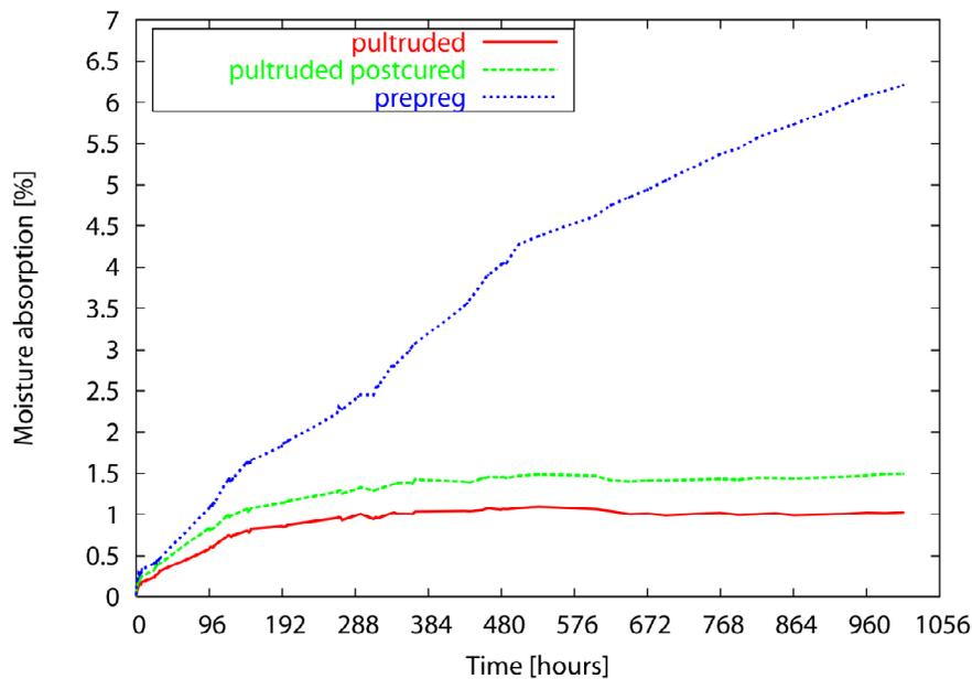
Figure 3. The results of moisture absorption tests on pultruded carbon fibre epoxy specimen (as received and with an additional post-cure) and autoclave cured carbon fibre epoxy prepreg.
