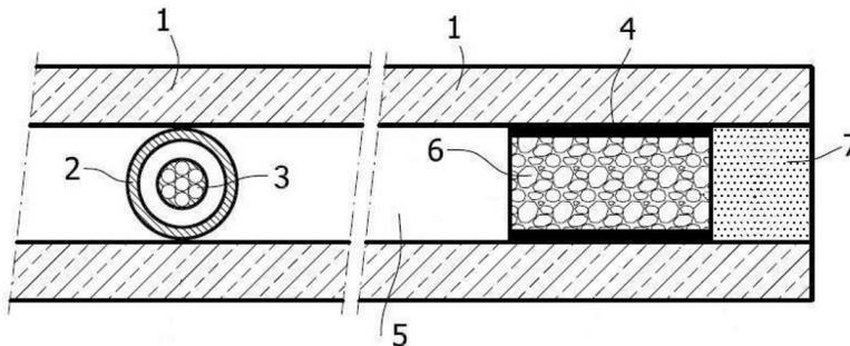
Figure 2. Cross-sectional view A-A' of the insulating glass panel, see Figure 1 for the total view, with (1) the glass plate, (2) the carbon tube, (3) the aramid cable, (4) the butyl sealant, (5) the argon filled double glass inner space, (6) the carbon spacer, and (7) the silicone structural adhesive.
