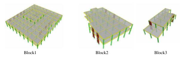
Fig 1. 3D modelling of sturctres in Etabs
