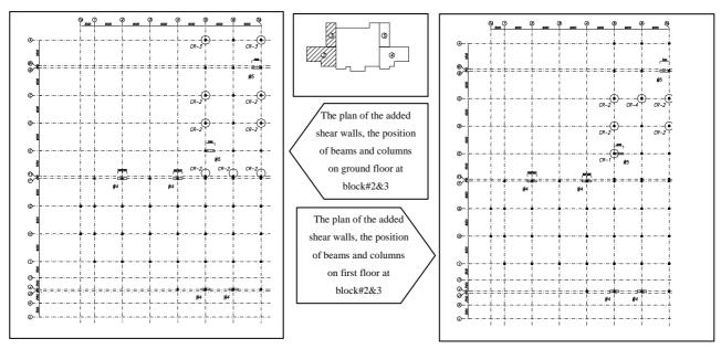
Fig 4. Locataion plan of Retrofitting shear wall, column , beams at block 2,3
