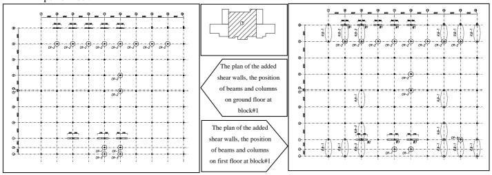
Fig 3. Locataion plan of Retrofitting shear wall, column , beams at block1
