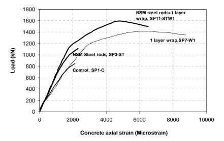
Figure 6. Load carrying capacity – axial strains relationship of SP1-C, SP3-ST, SP7-W1 and SP11-STW1
