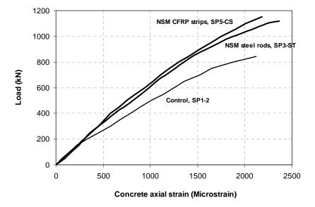
Figure 5. Load carrying capacity – axial strains relationship of SP1-C, SP3-ST, SP5-CS
