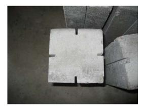
Figure 3b. four slits each of dimensions 18 x 5 mm for specimens strengthened by four exterior CFRP slotted strips.
