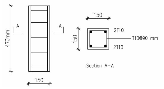
Figure 2. Columns dimensions and reinforcement.
