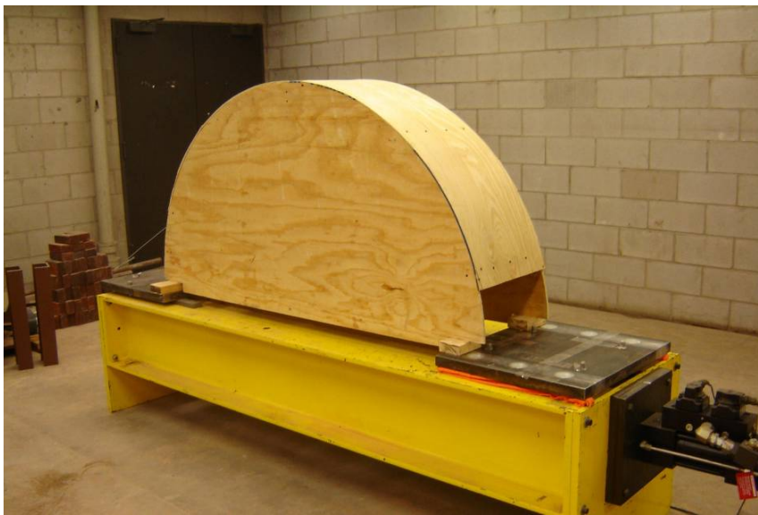
Figure 10. Wooden Frame for Masonry Arch Fabrication.
