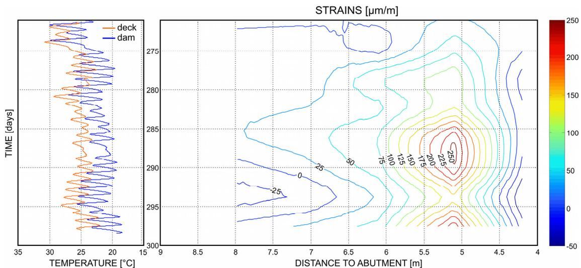
Figure 5. Strain field as function of distance to abutment and time for top FOS layer
