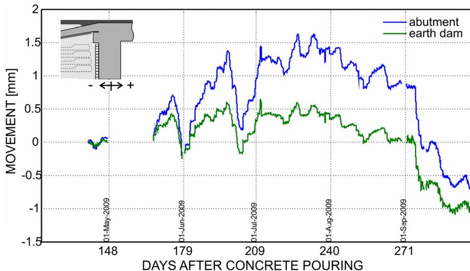
Figure 4. Movement of abutment vs. earth dam over time
