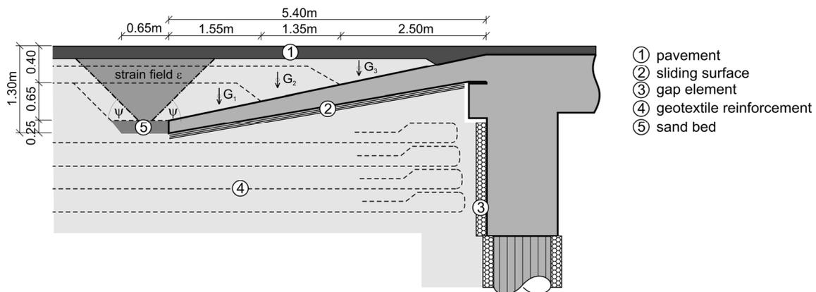
Figure 2. Approach slab detail of Marktwasser Bridge
