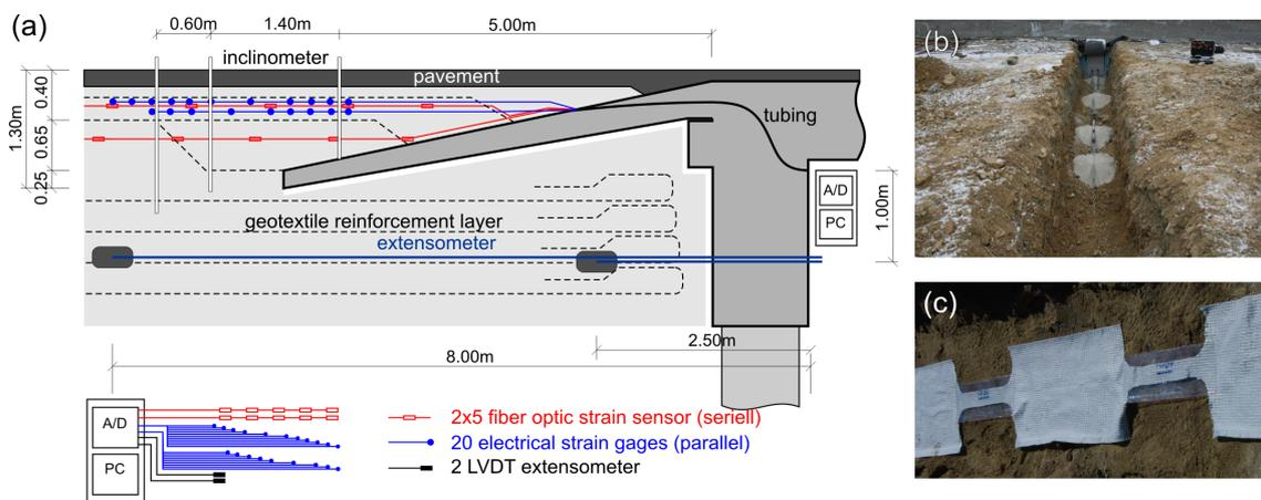
Figure 3. (a) Instrumentation of southern abutment and dam, (b) Installation of extensometer, (c) Installation of geotextile based fiber optic strain sensors
