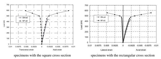
Figure 4. Load-strain relationships of the concentrically loaded columns
