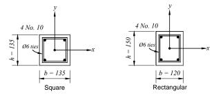
Figure 1. Cross sections shapes
