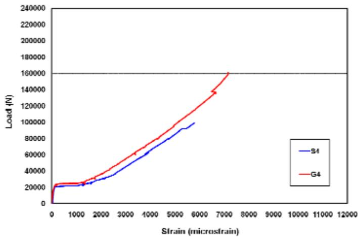
Figure 10. Comparison between the sensors S4 and strain gauges G4.
