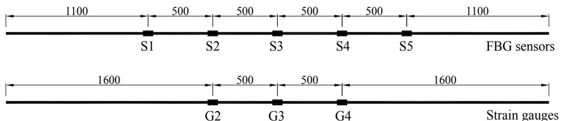
Figure 2. Locations of the FBG sensors and electrical resistance strain gauges on the V-ROD GFRP bars No. 6 and 8.
