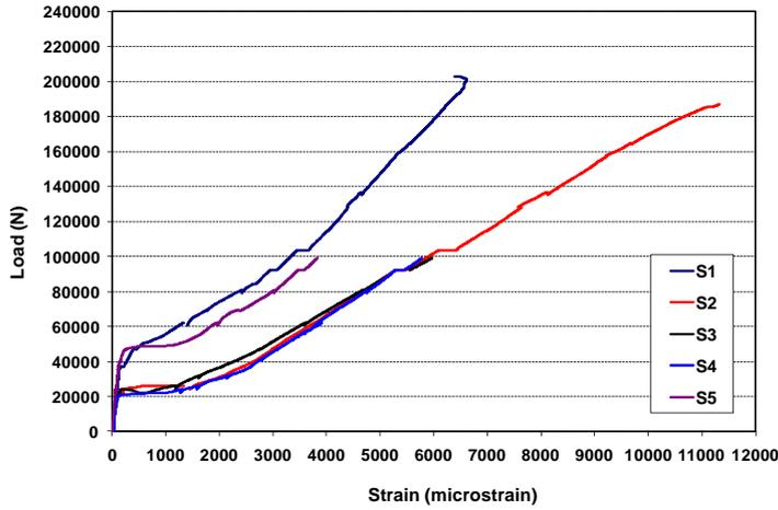
Figure 6. Load-strains relationship using the FBG sensors.
