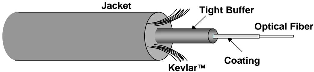
Figure 1. Optical cable basic construction (Diagram not to scale).
