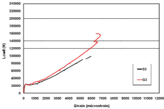
Figure 9. Comparison between the sensors S3 and strain gauges G3.
