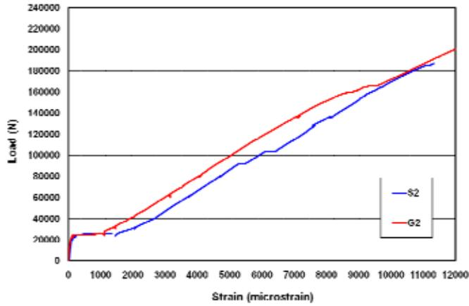
Figure 8. Comparison between the sensors S2 and strain gauges G2.
