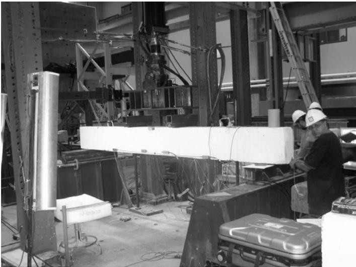
Figure 5. Test setup for beam testing.
