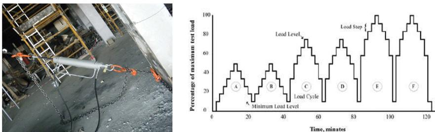
Figure 3. Load testing: (a) Hydraulic jack; (b) Load cycles as per ACI 437.1R-07.
