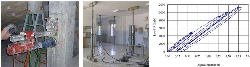
Figure 7. (a) Concrete core sampling; (b) Static load test; (c) Hysteresis diagram example.
