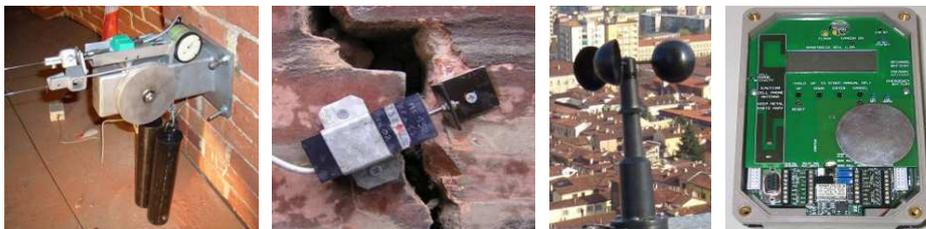
Figure 4. Monitoring devices: (a) Displacement transducer; (b) Crack transducer ; (c) Wind anemometer; (d) Smart Brick® device.
