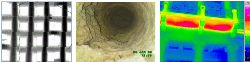
Figure 1. Captures from: (a) Ferroskan, (b) Videoendoscopy, (c) Thermocamera.
