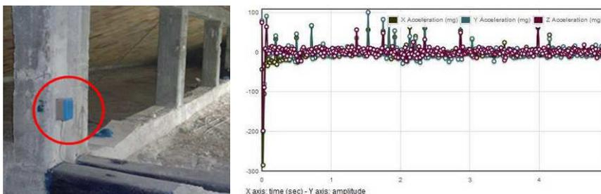
Figure 8. (a) Smart Brick® installed at roof level; (b) Acceleration recorded during seismic event.
