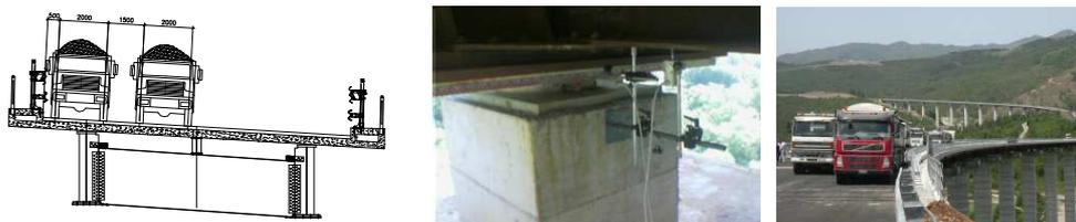
Figure 10. (a) Loading scheme; (b) Displacement transducer at the support; (c) View of the road.
