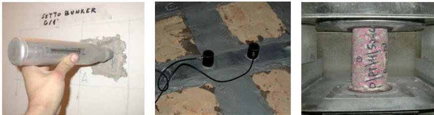
Figure 2. Material testing: (a) Rebound hammer; (b) Ultrasonic survey; (c) Concrete core testing.
