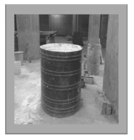
Fig 4 Container for Casting Concrete
