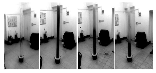
Fig 1 Test Setup showing test tube filled with water and sedimentation process of cement paste (Phase I)
