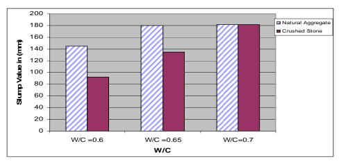
Fig 5 Average Slump Value for Natural Agg. And Crushed Stone
