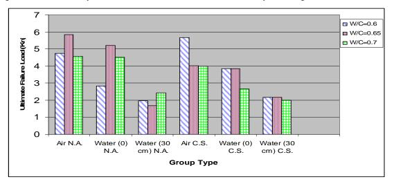
Fig 8 Flexure strength of beams after 28days
