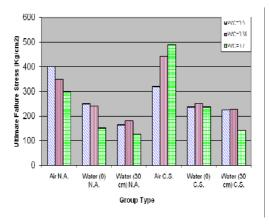
Fig 6 Compressive strength of after 7 days
