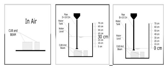
Fig 2 A Schematic Diagram showing method of casting concrete. Phase 2
