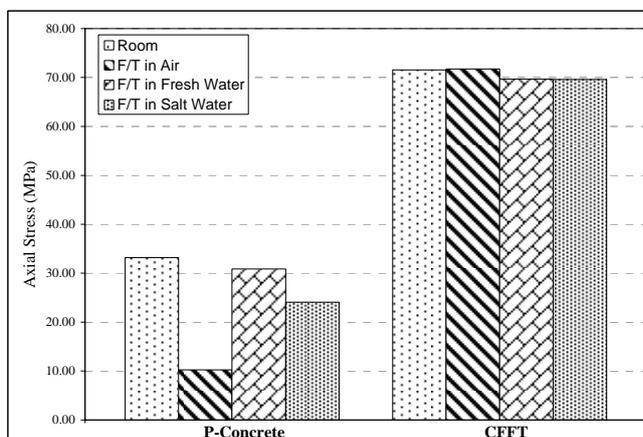
Figure 6. Compressive stress of unconfined and confined (conditioned and unconditioned) specimens.
