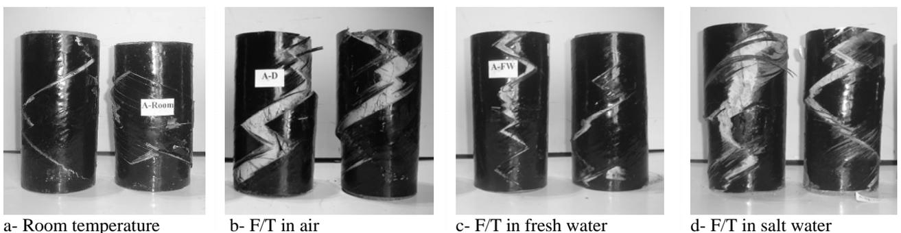
Figure 8. Failure modes of conditioned and unconditioned CFFT cylinders.
