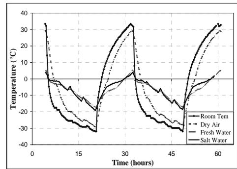
Figure 3. Temperature variation inside the specimens during two complete F/T cycles.
