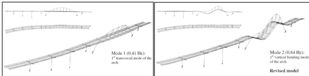
Figure 7. First and second modes of vibration.
