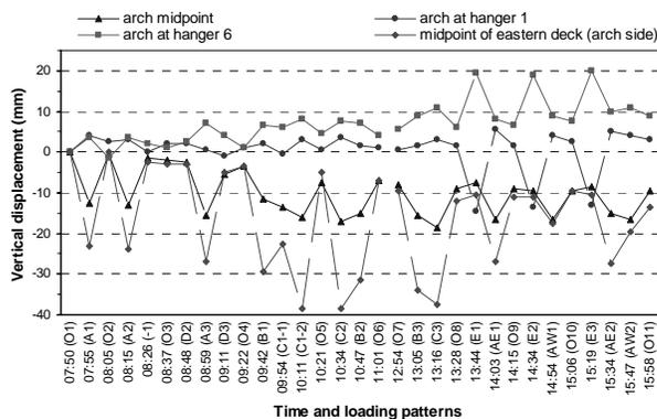
Figure 5. Arch and bridge deck vertical displacements. Hanger 1 corresponds to arch 1/4-point on Swedish side and hanger 6 to arch 1/4-point on Norwegian side.
