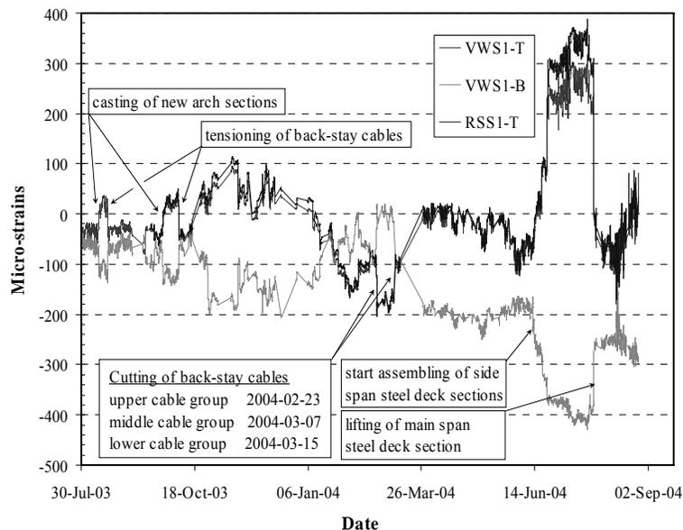
Figure 3. The above figure shows how the work on site is mirrored by the measured strains. The gauges are installed at the top and bottom of arch segment S1 close to the arch base on the Swedish side. VWS1-T vibrating-wire gauge at the top of S1, VWS1-B vibrating-wire gauge at the bottom of S1, RSS1-T resistance strain gauge at the top of S1.
