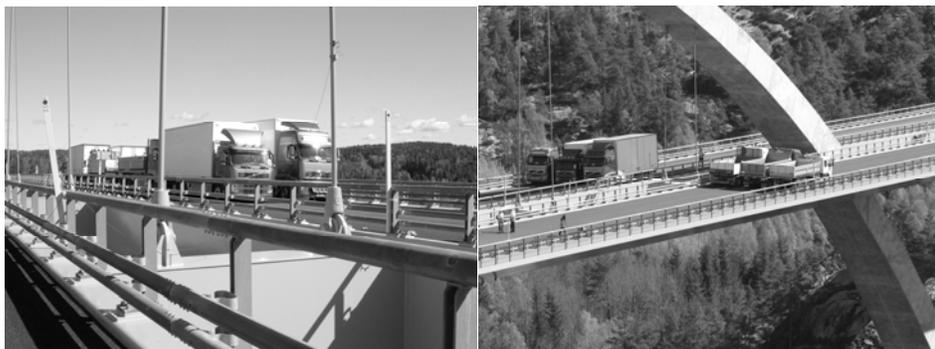
Figure 4. Loading pattern C with 8 lorries (left photo) and loading pattern E with 6 lorries (right photo).
