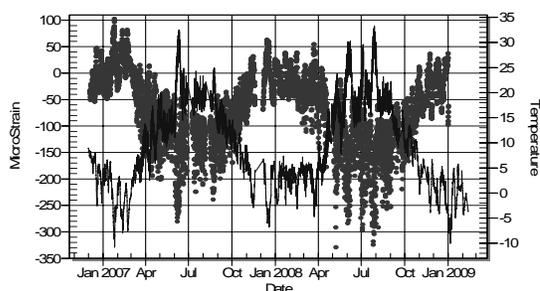
Figure 6. Temperature effect (solid line) on the strain (dotted) at top of arch segment S1.
