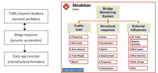
Figure 4. Left: Schematic representation of the relationship between traffic induced vibrations and its effect on early-age concrete; Right: Structure of the bridge monitoring system.
