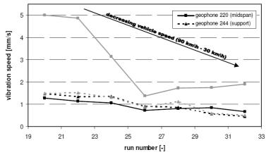
Figure 7. Influence of the velocity of the vehicle on the magnitude of bridge vibration (acceleration) for different runs, while reducing the velocity from 90 km/h to 30 km/h.
