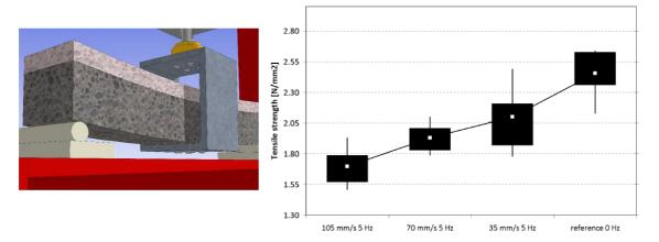
Figure 8. Left: Impression of the test setup; Right: Tensile strength versus different dynamic loadings.
