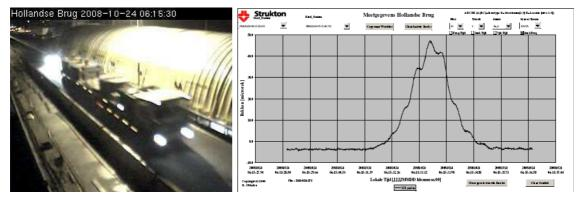
Figure 6. Left: Image of ballast truck 100 mT; Right: Strain registration of main girder during passing.
