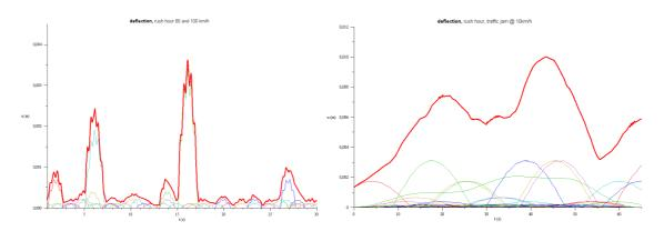
Figure 3. Left: Case 1) Typical deflection during intensive traffic including heavy cargo vehicles; Right: Case 2) Typical deflection during congestion.
