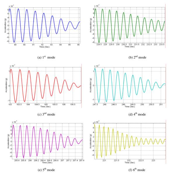
Figure 5. Eliminating initial displacements and ambient vibration loads from records using RDT
