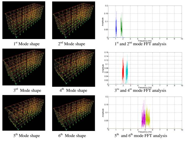
Figure 4. First six structural mode shapes and FFT analysis results
