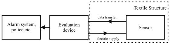
Figure 3: Principle operation of monitoring systems
