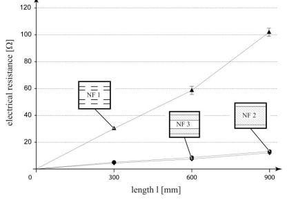
Figure 5: Electrical resistances of narrow fabrics
