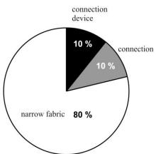
Figure 6: Percentage of connection parts of the overall electrical resistance
