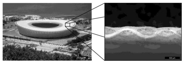
Figure 1: World Cup soccer stadium in Cape Town, SA (left) and microscopic cross section of used PTFE-coated glass fabric (right)
