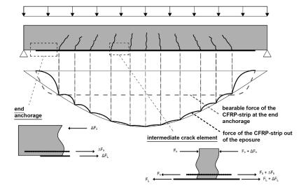
Figure 3. Principle of the bond force transfer of externally bonded FRP
