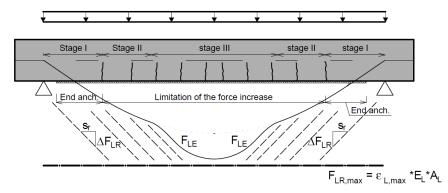
Figure 4. Concept of the simplified approach
