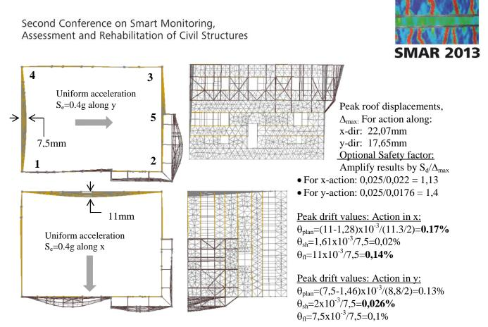
Figure 5: Deformed structure under uniform acceler. according to the proposed method. Critical is action in x
