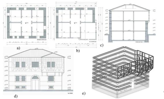
Figure 3: Representative sample building from the historical city core of Xanthi. (a) Plan view of first floor, (b) Plan view of upper floor, (c) Building cross section, (d) Front view, (e) Arrangement of timber laces
