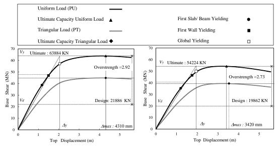
Figure 4. Sample of the capacity curves of the M1 (left) and M5 (right) buildings.
