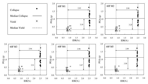
Figure 5. IDA results at yield and collapse along with collapse-to-yield PGA and IDR ratios.
