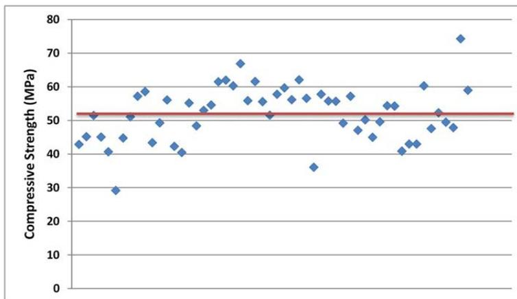
Figure 3. Compressive Strength in different parts of the jetty
