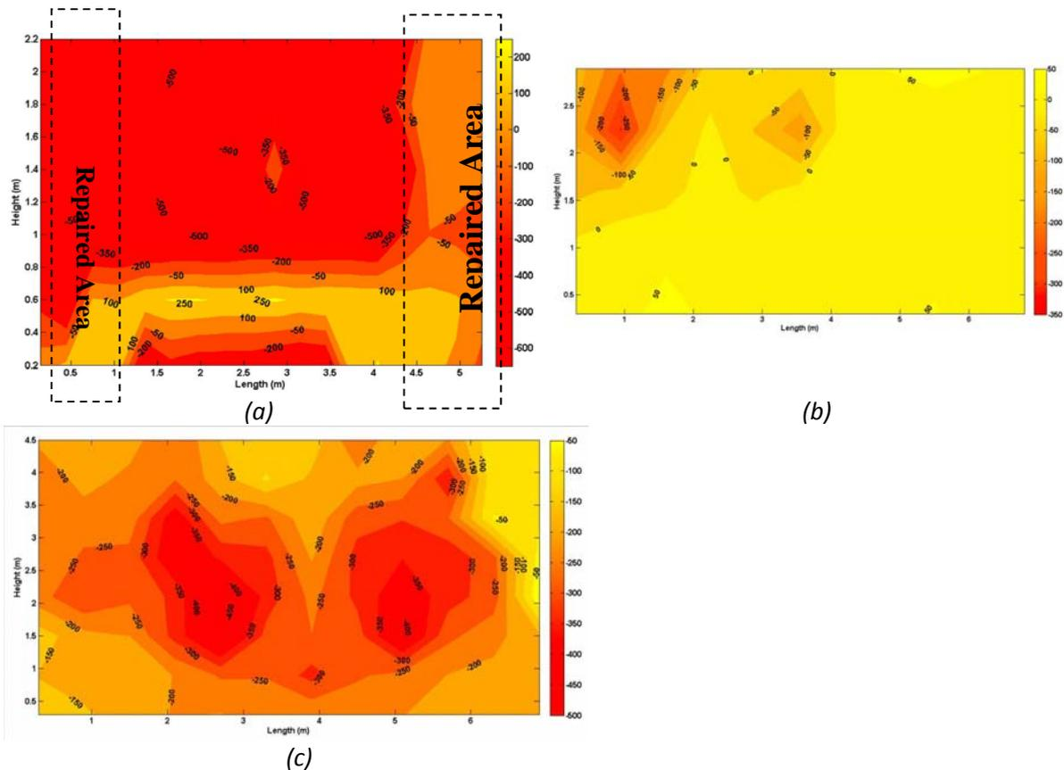
Figure 7. Half-cell potential contours (mV) in a) bottom of a beam near the coast, b) an area on channel bridge, c) an area on uploading pier
