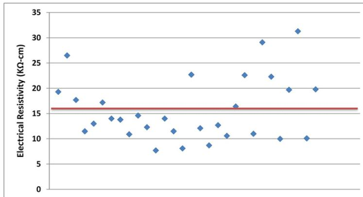
Figure 5. Electrical resistivity of concrete cores in different parts of the jetty
