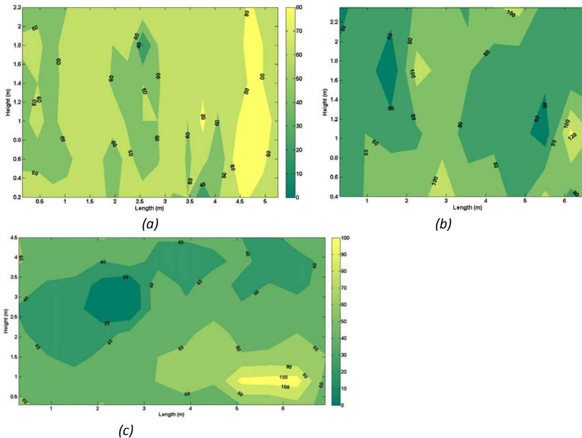
Fig. 6. Cover thickness (mm) in a) bottom of a beam near the coast, b) an area on channel bridge, c) an area on unloading pier
