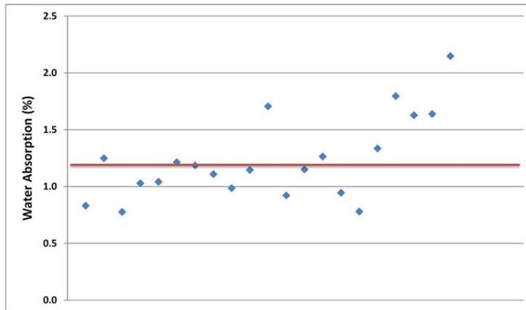
Figure 4. 30 minutes water absorption in different parts of the jetty
