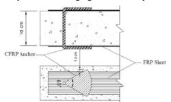
Figure 3. CFRP Anchor with a fan in one direction.
