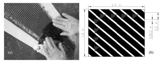
Figure 7. (a) Application and (b) design location of the of CFRP anchors on panel specimen
