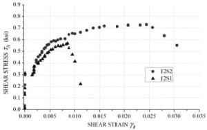
Figure 9. Shear stress and strain curve for specimen F2S1&F2S2.
