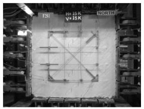
Figure 6. Instrumentation of Panel Element
