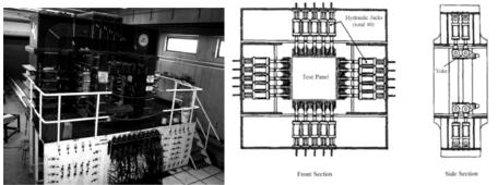
Figure 4. Illustration of load application by in plane hydraulic jacks (Hsu et. al., 1995)
