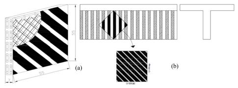
Figure 5. (a) Panel specimen, (b) The T-Beam idealized as an assemblage of membrane elements.
