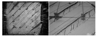
Figure 8. (a) Debonding of FRP sheets in panel F2S1, (b) Debonding and FRP rupture in panel F2S2
