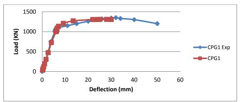
Fig. 6 Load- deflection curve of CPG1
