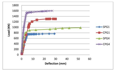
Fig. 10 Effect of web aspect ratio
