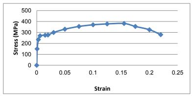
Fig. 3 Stress-strain diagram of steel
