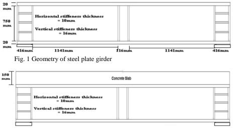
Fig. 2 Geometry of composite plate girder
