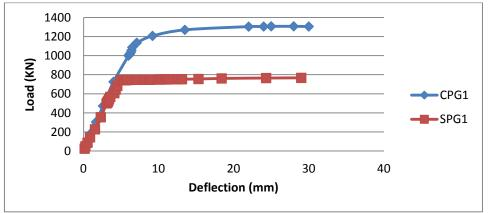
Fig. 8 Load-Deflection curve for composite and plate girders
