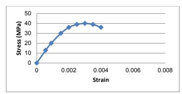
Fig. 4 Stress-strain diagram of concrete
