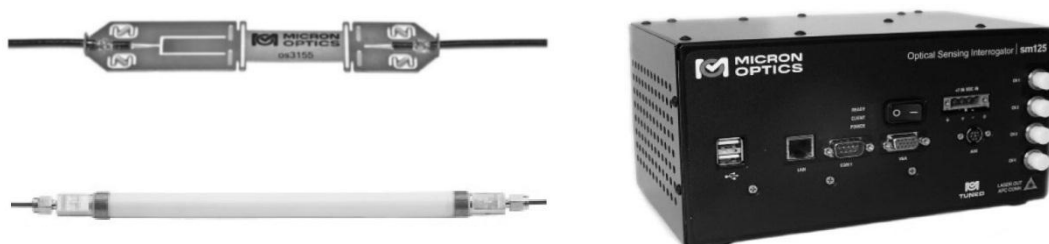
Figure 5. Instruments used for measuring strain in the Jeesiöjoki Bridge. Above left, the os3155 sensor and below it the os3600 sensor. The SM125-500 interrogator is on the right. The photographs are not to scale.
