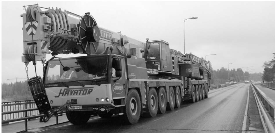
Figure 6. Bridge loading using two vehicle cranes parked tail-to-tail.
