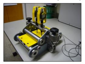
Figure 2. Portable 4-point bending test facility for strain calibration in the test field area (designed by H. Kohlhoff, BAM).
