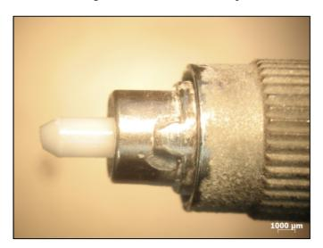
Figure 4. Connector corroded by salt-water influence during salt-water attack test.
