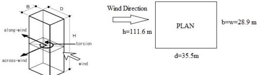
Figure 3. Definition of wind direction
