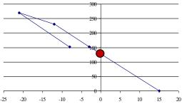
Figure 14. Load history during the hole drilling in terms of strains (vertical axes) vs number of readings
