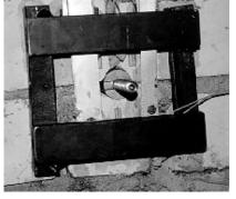
Figure 7. Dilatometer test on the masonry
