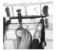
Figure 6. Flat jack test on the masonry
