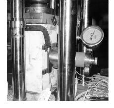
Figure 4. Dilatometer view inside the brick hole
