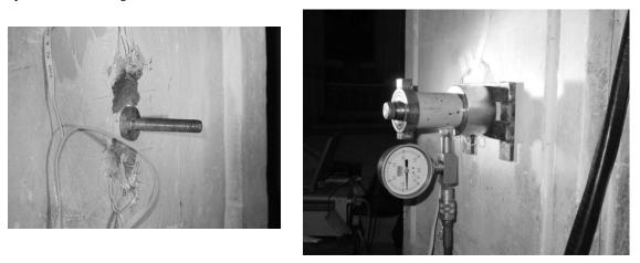
Figure 11. Instrument disposition in the hole and test equipment for the load measurement
