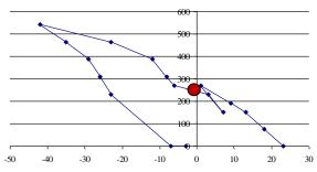
$\begin{array}{ll} Figure 13. & Load [kN] strains [\mu m/m] \\ curve for SG1 in D1 pillar \end{array}$
