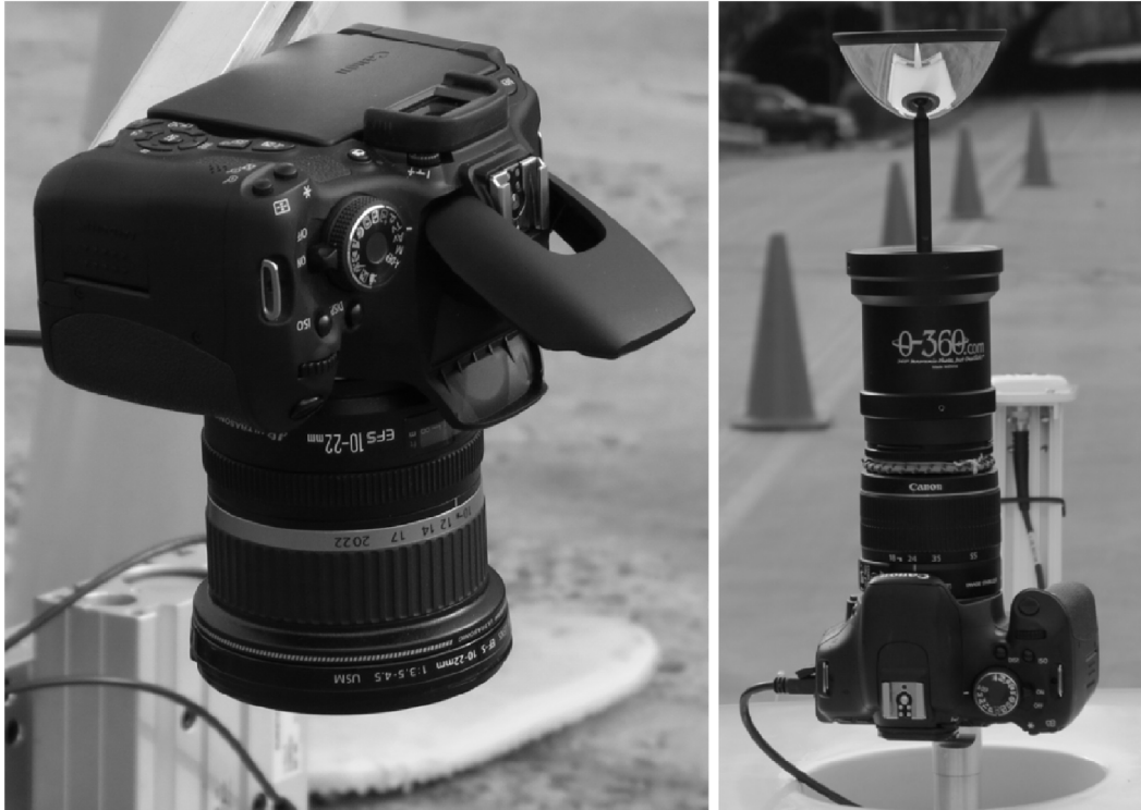
Figure 3. High resolution deck surface imaging camera (left) and the camera with 360 degree mirror for panoramic imaging (right).
