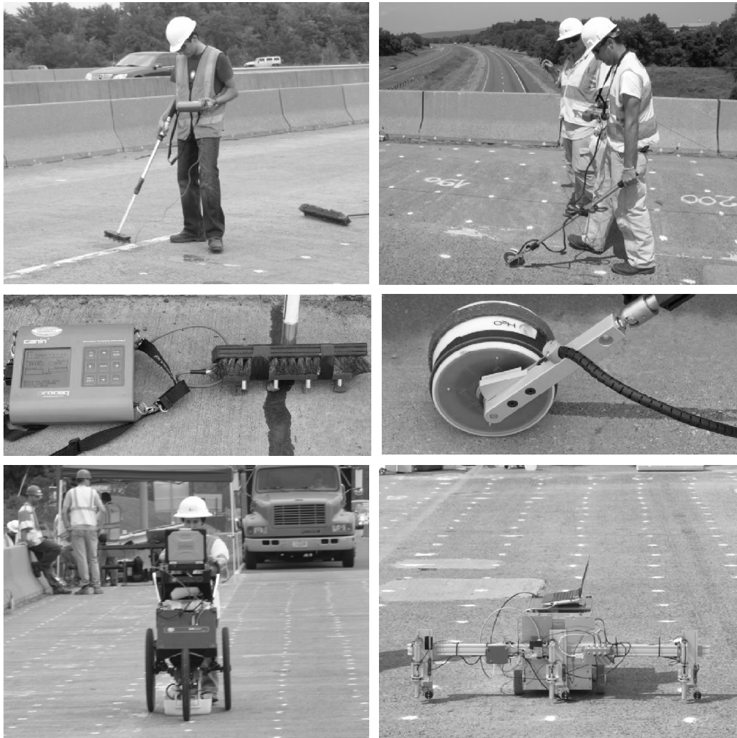
Figure 1. NDE technologies: Electrical resistivity measurement (top left) and probe (middle left), half-cell potential measurement (top right) and probe (middle right), GPR measurement (bottom left) and impact echo testing using Stepper (bottom right).
