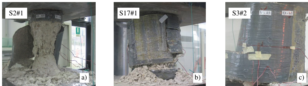
Figure 6. Typical failure modes of SFRP confined specimens.
