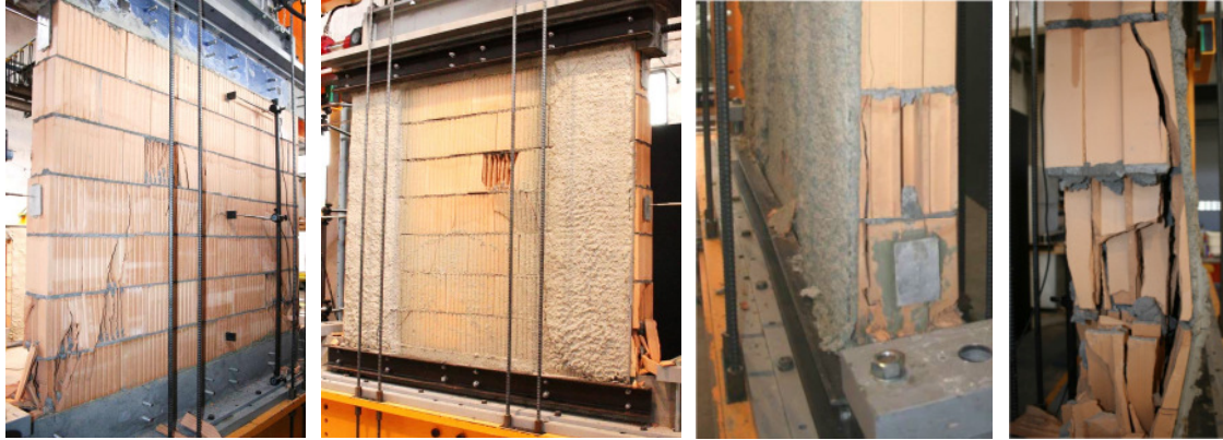
Figures 4a to 4d: Failed specimens in Series MR-C. a and b: MR-C2, c: MR-C3, d: MR-C5 (from left to right)
