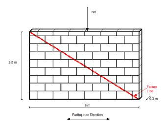
Figure 4. Wall subjected to in-plane load
