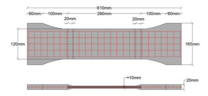
Figure 1. Configuration of coupons (Triantafillou 2012a).
