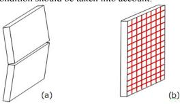
Figure 3. (a) Vertical flexural failure, (b) strengthening by TRM System (Triantafillou 2012b).
