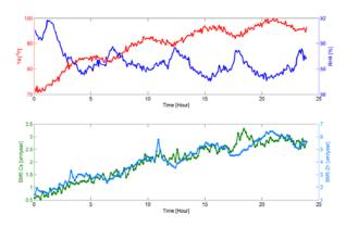
Fig 5. A direct data plot of temperature /humidity internal sensor (top) and corrosion bimetallic sensor (bottom) showing direct correlation between temperature, humidity and corrosion rate.
