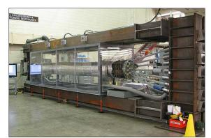
Figure 3. Full scale cable mock-up, 6m long and 0.5m in diameter under tension is encased within a custom made corrosion chamber
