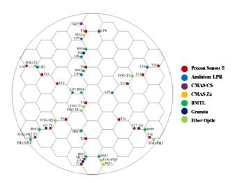
Figure. 2. A schematic drawing of cable cross section showing the embedded Precon temperature/humidity sensors and LPR/CMAS corrosion sensors and their distribution
