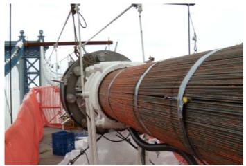
Fig. 9. View of indirect sensing sensors installed within the main cable at 4 groove positions and the direct sensing Main Flux scanner near the cable band.
