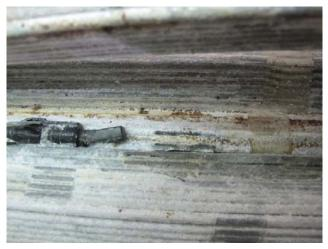
Fig. 6. View of cable mockup during the after completing the test showing a temperature, humidity sensors which survived the harsh environmental test and compaction.
