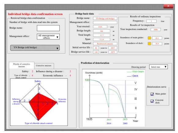
Figure 8. Sample screen of an optimum maintenance plan for YN Bridge
