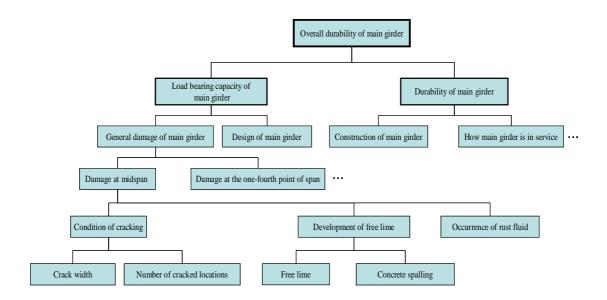
Figure 2. Part of the process of evaluating overall durability of main girder
