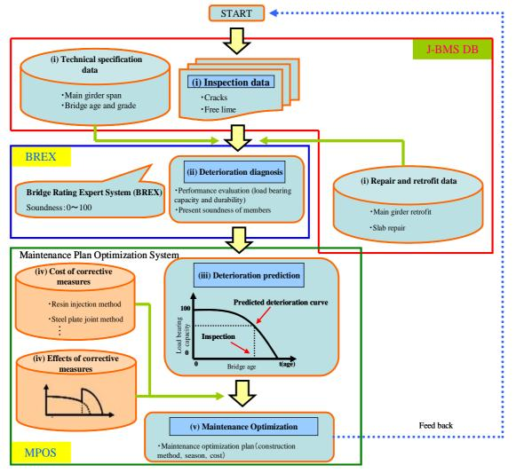
Figure 1. Configuration of J-BMS
