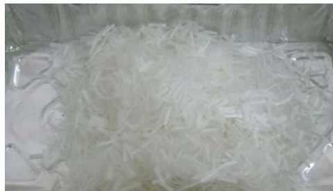
Figure 2. PVA fiber used in experimental study.
