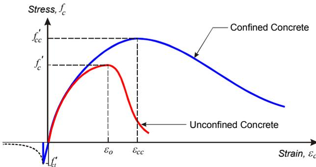
Figure 4. Effect of the full FRP wrapping on concrete behaviour
