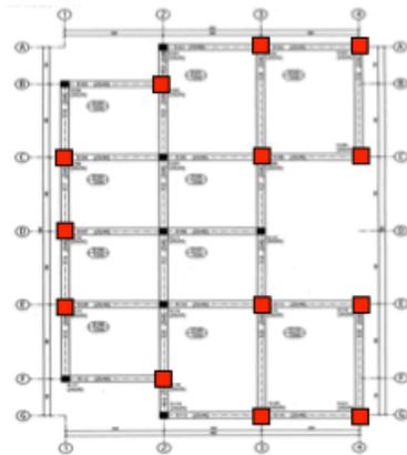
Figure 5. Scheme of the column concrete jacketing used in this study
