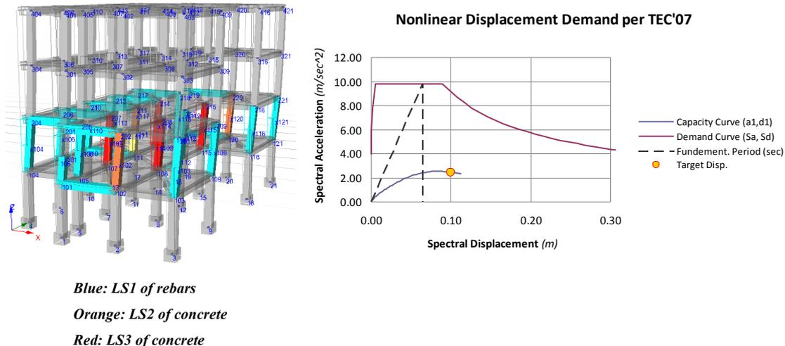
Figure 3. Damage distribution when the target displacement is reached (left), and the definition of the target displacement as per TEC (right) before FRP wrapping
