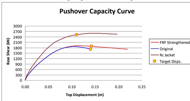
Figure 8. Comparison of the pushover capacity curves for 3 cases
