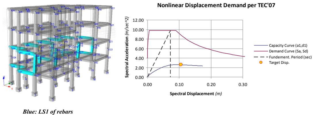
Figure 6. Damage distribution when the target displacement is reached (left), and the definition of the target displacement as per TEC (right) after FRP wrapping
