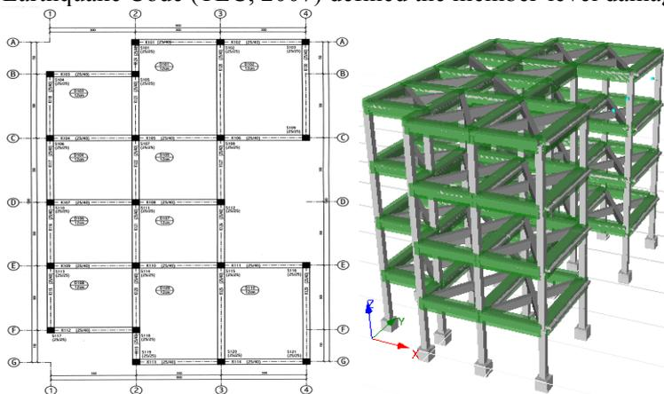
Figure 2. Formwork plan of the structure (left) and 3D view of the SeismoStruct model (right), details of which can be found in Başaran (2006)
