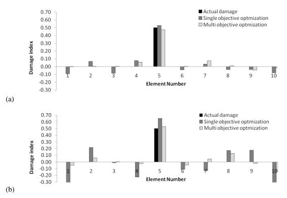
Figure 3. Damage severity estimation for element No. 5 : (a) 5% noise level, and (b) 20% noise level.
